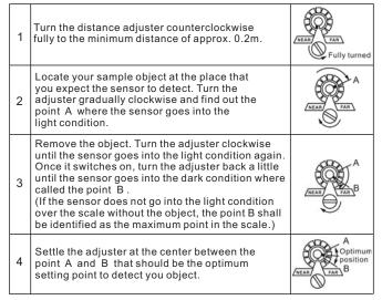
(\*1): Turn the distance adjuster gradually and lightly with the  $\,$  attached  $\,$ screwdriver. If the distance adjuster is over-turned or pressed heavily, it may be damaged.
