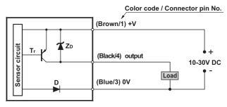
Symbol...D: Reverse polarity protection diode.
