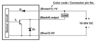
Symbol...D: Reverse polarity protection diode.
